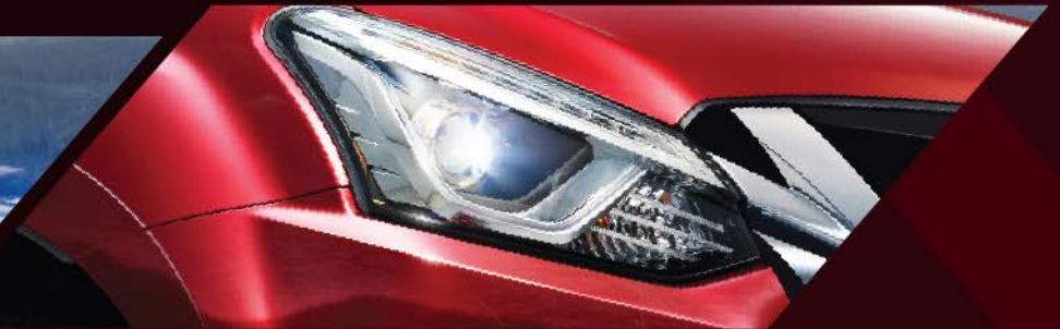
Bi - LED Auto - levelling Headlamps with DRL
