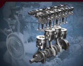
Diamond-like Carbon-coated Pistons and Injectors
