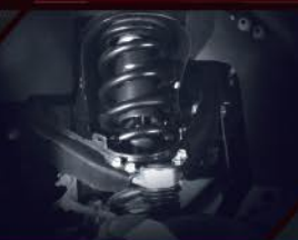
Front Independent Double Wishbone Coil Suspension with Stabilizer Bar
