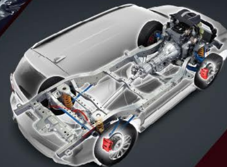
Heavy - duty Ladder Construction Chassis
