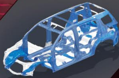
High Tensile Steel Body Construction with Tailor-welded Blanks and Side Anti-intrusion Bars
